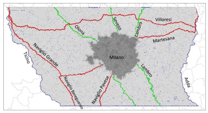
Fig. 1 - Numerical flow model implemented using a Voronoi mesh. Rivers inside the model are represented in green (in blue the ones at the bouondary: Ticino and Adda), channels are shown in red while blue points are wells.
