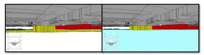
Fig. 1 - On the left, the database information is implemented in ArcGIS Pro: the elements in grey represent the bottom of superficial buildings, whose information derives from the DBT (Topographic DataBase); the yellow element is the M3 line at Duomo station; the red one is the M1 line at Duomo; on the right, the superimposition of Modflow-USG outputs in ArcGIS Pro at Duomo stations is visible in light blue.
