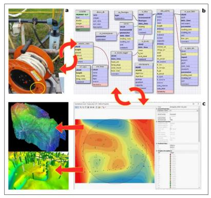
Fig. 1 - a. Broken phreatimeter with 1 m of cable missing (not always recorded by the field operator); b. default structure of the Midvatten SQLite DB (open source QGIS plugin); c. final results of data processing.
