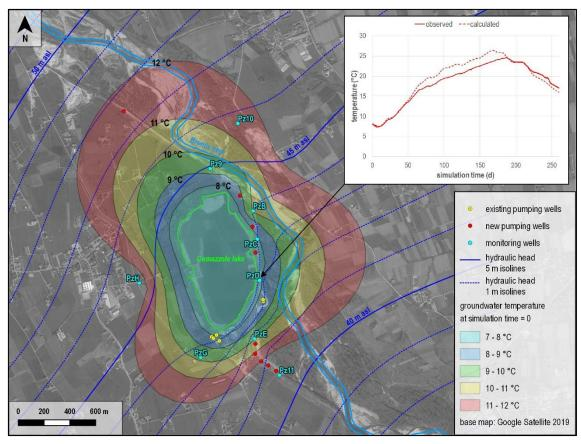
Fig. 5 - Initial distribution of groundwater temperature around the Camazzole lake and transient simulation results in PzD monitoring well during the first period of groundwater exploitation
