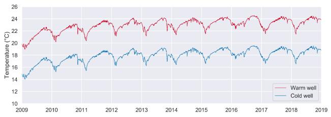
Fig. 1 - Simulated groundwater temperature evolution at the ATES wells (warm and cold wells) over the 10 years simulation period.
