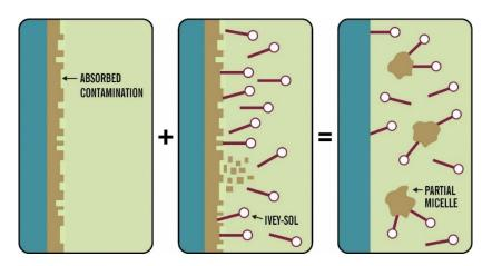
Fig. 1 - Operating principle of Ivey-sol® surfactants
