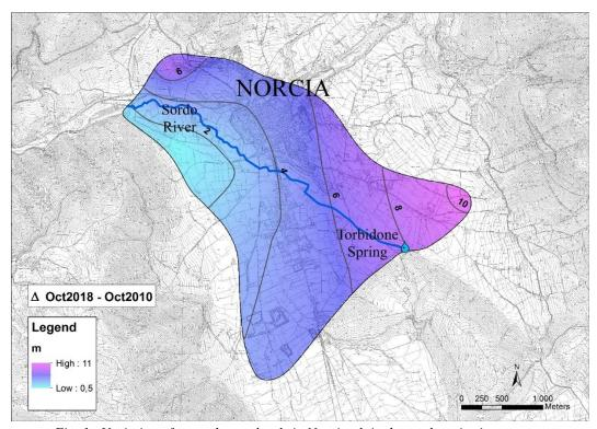
Fig. 1 - Variation of groundwater levels in Norcia plain due to the seismic sequence
