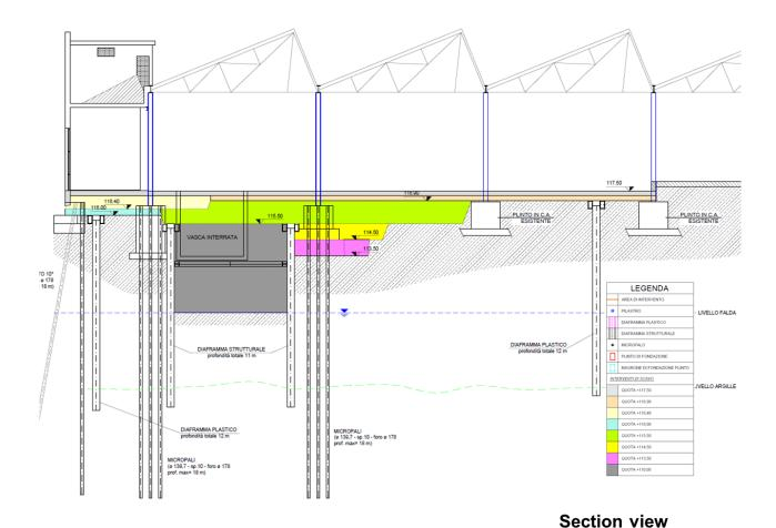
Fig. 1 - Section view of the realized physical containment
