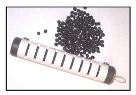
Fig. 1 - Bio-Trap® sampler from Microbial Insights, Inc.
